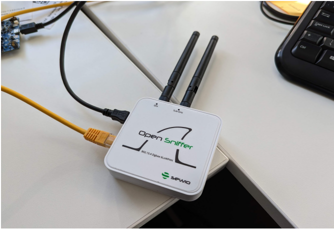
Fig. 5: A Sewio OpenSniffer is utilised for packet capture and injection.
